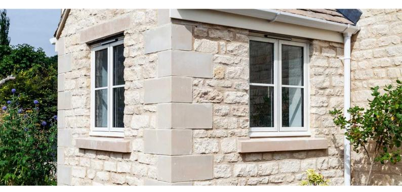
The Alitherm 800 aluminium flush casement window in terms of performance, offers an 'A' rating for energy efficiency. Smart's polyamide thermal break technology and the correct sealed unit means that the flush casement can achieve U-values as low as 1.3 W/m²K. They achieve PAS 24:2012 security and are rigorously tested for water, air, and wind resistance.
