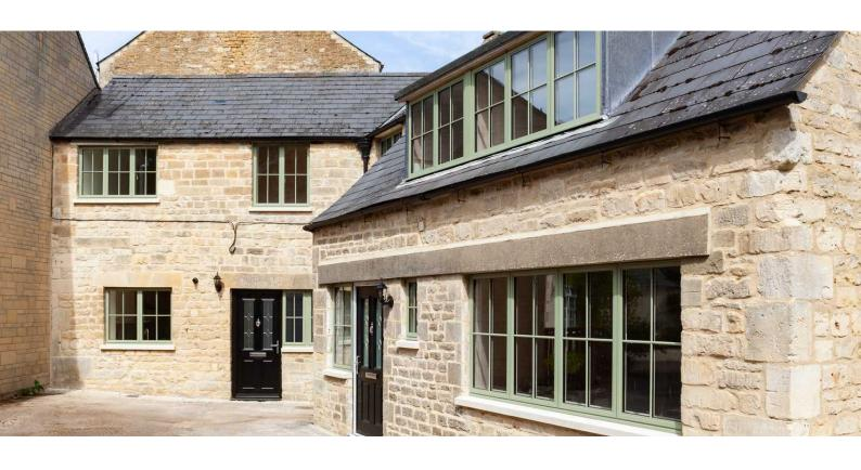
Our aluminium flush casement is fabricated using Smarts Alitherm 800 profile. Aesthetically, the flush casement windows sit flat with the outside frame, providing a completely flush exterior that is typically associated with traditional timber windows. Featuring slim lines with ultra-slim transoms and mullions, the flush casement makes for a perfect option in both traditional and high-end contemporary applications.
